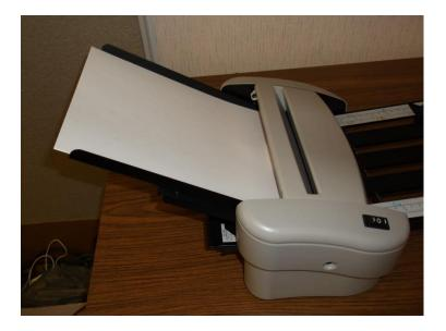
When you use the bypass, only insert paper if the machine is at rest (the rollers cannot be turning).
