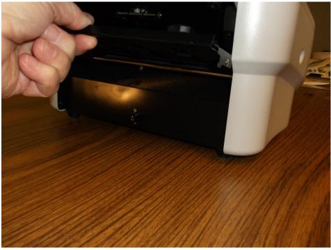
Fold tables must be inserted over the top of the silver bar. NEVER under the silver bar.
